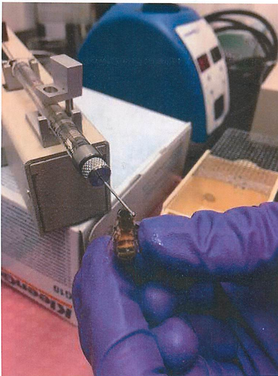
Figure A4.1. A newly-emerged worker bee is topically treated 1 \mu l of tested compound using Hamilton micro syringe in a precision micro-applicator. Once treated, the bees were placed in plastic cages and fed one sugar cube. The bees were incubated at 33°C for 24 hours. Bee mortality was assessed 24 h post-treatment. In this test, LD50 and bee mortality were assessed.
