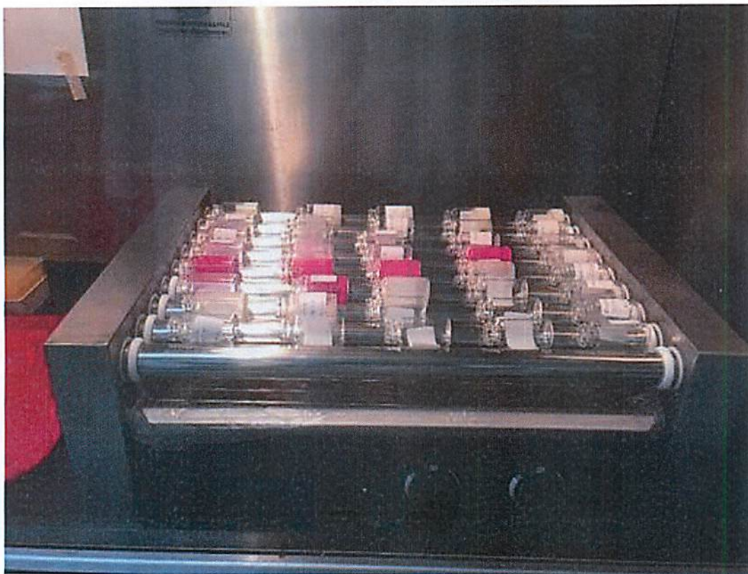
Figure A4.2. Treated scintillation glass vials are rotated on a cold hot dog roller under the fume hood at room temperature for 2-3 h until the solvents are completely evaporated and compounds are homogenously spread on the inner surface of vials.
