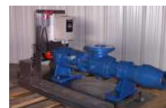
Figure 25: Honey Pump, 3" Progressive Cavity, Variable Speed Drive (cowenmfg.com)
